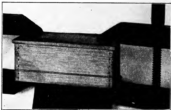
Fig. 295—Box in Position for Nailing
